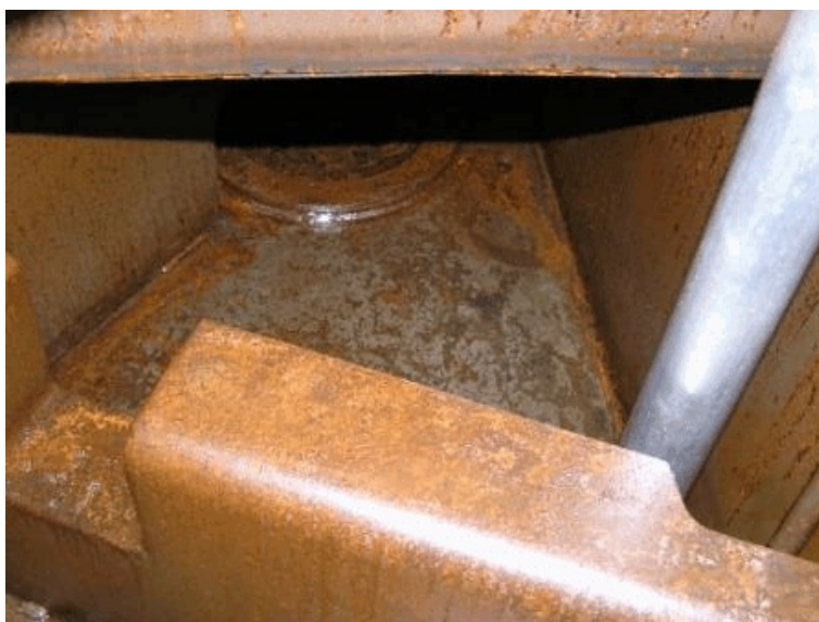
Corrosion inside vehicle tank
