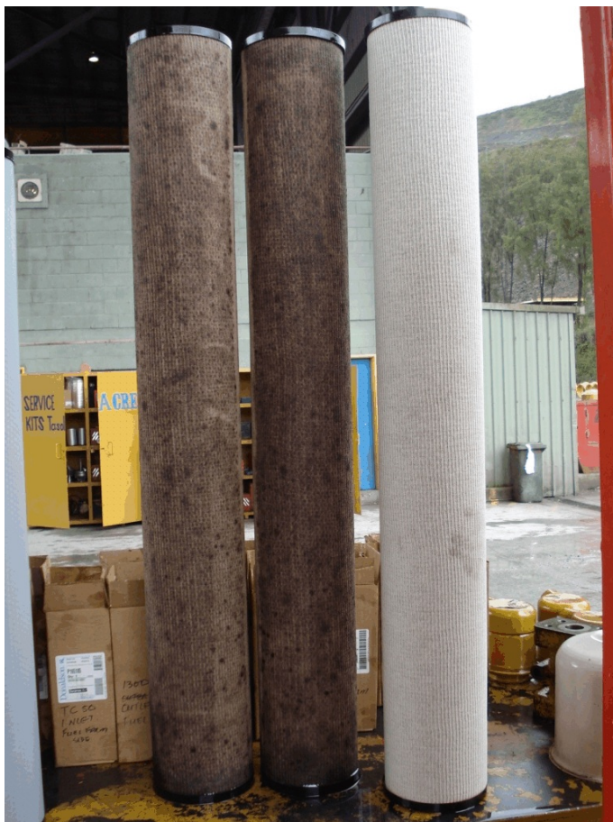
Filters from untreated and treated fuel
